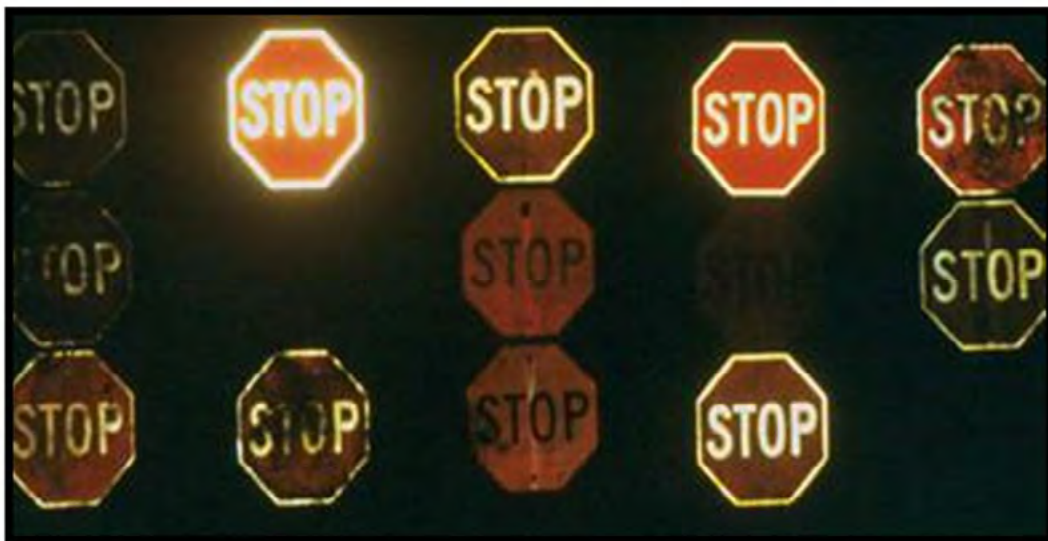
Nighttime view - Notice the difference in visibility per sign during nighttime
