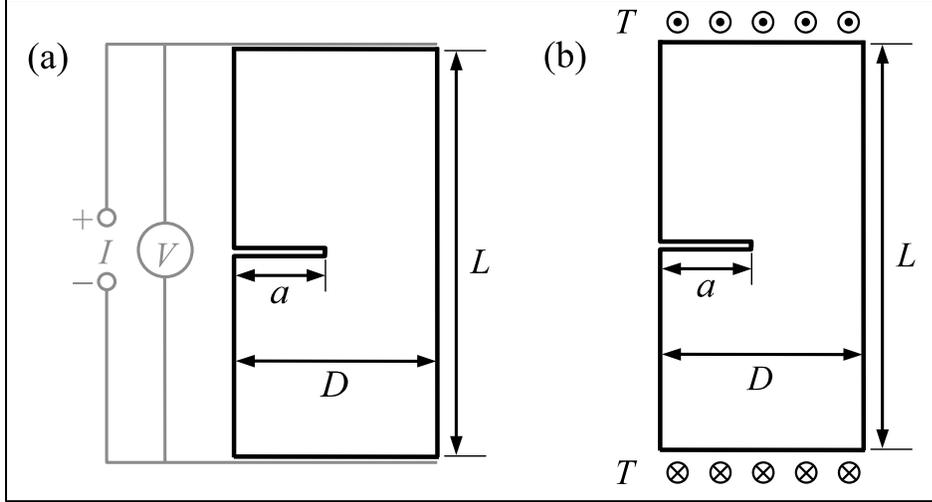
**Figure 4.1: A damaged specimen with notch length  $a$ : (a) crack detection with conductive plates attached to the ends of the specimen; (b) mathematical analogy of anti-plane shear applied to the ends of the specimen.**
