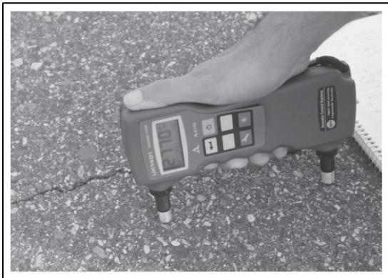
**Figure 2.1: Ultrasonic tester UK1401. (Khazanovich *et. al.*, 2005)**
