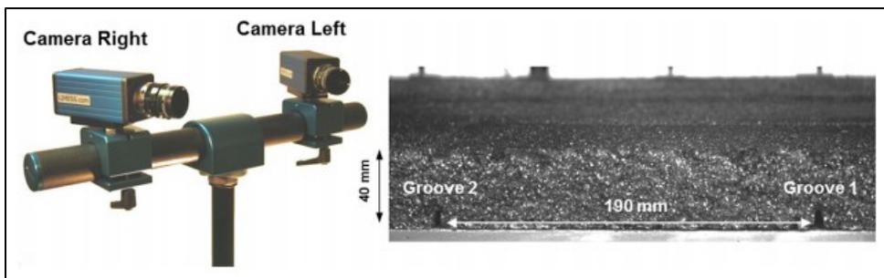
**Figure 2.6: Setup for Digital Image Correlation system (left). Real image of the lateral surface of a test slab (right) (Bueno & Arrigada, 2016).**
