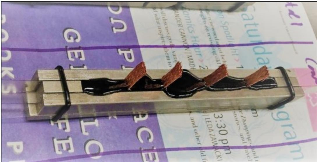
**Figure 3.6: Sample with copper electrodes immediately after pouring.**
