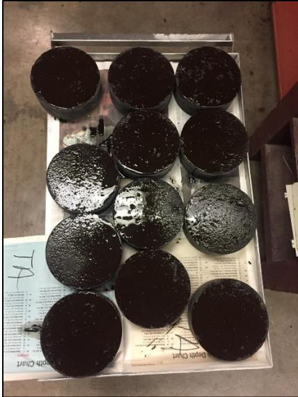
**Figure 6.1: Bottom pucks with applied tack coat.**
