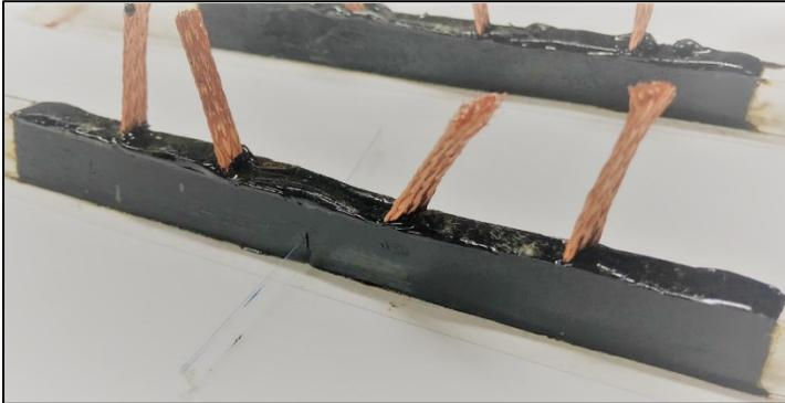
**Figure 4.4: Sample preparation: foil film holding the notch.**
