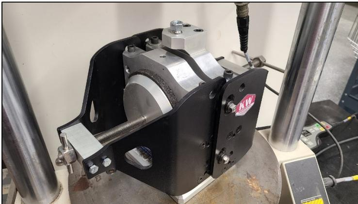
**Figure 6.5: MS-43 Asphalt Tack Bond Shear Strength Apparatus**
