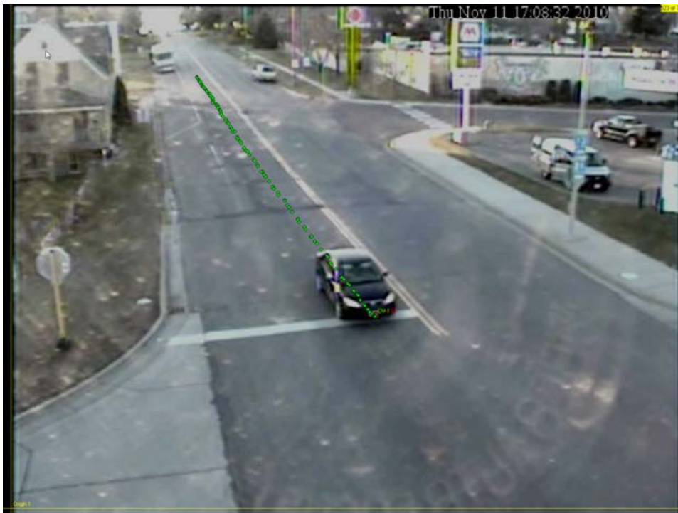
Figure 3.3 Screen Trajectory for an Example Vehicle, Measured Using Videopoint
