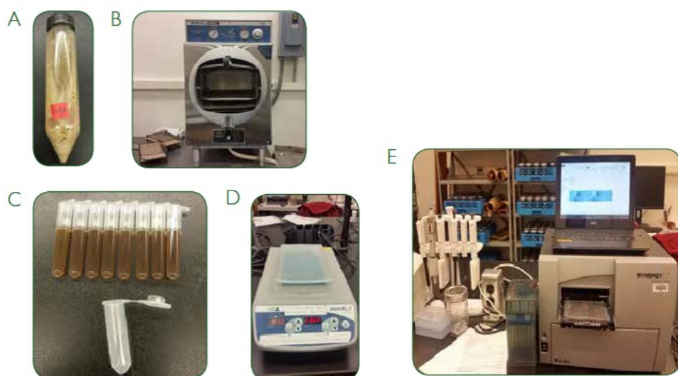
Figure 3.4 (a) Lab procedure for the ACE Protein Index, (b) glass tubes, (c) autoclave clarified extract, (d) protein assay, and (e) spectrophotometric plate reader. (Moebius-Clune et al., 2016)
