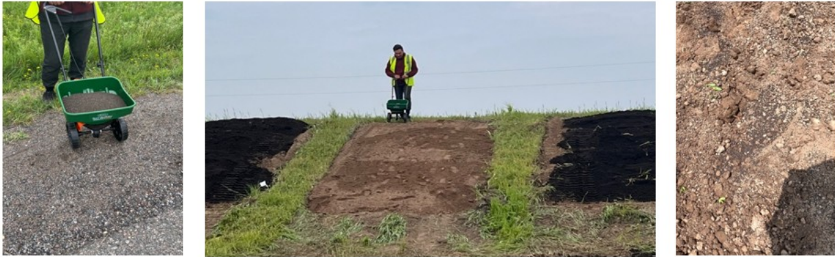
Figure 6.5 Distribution of proprietary amendment in PA plots with fertilizer spreader.
