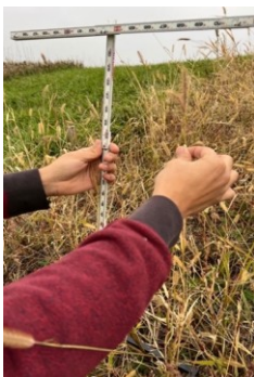
Figure 6.11 Grass height measurement procedure with ruler in the field plots.
