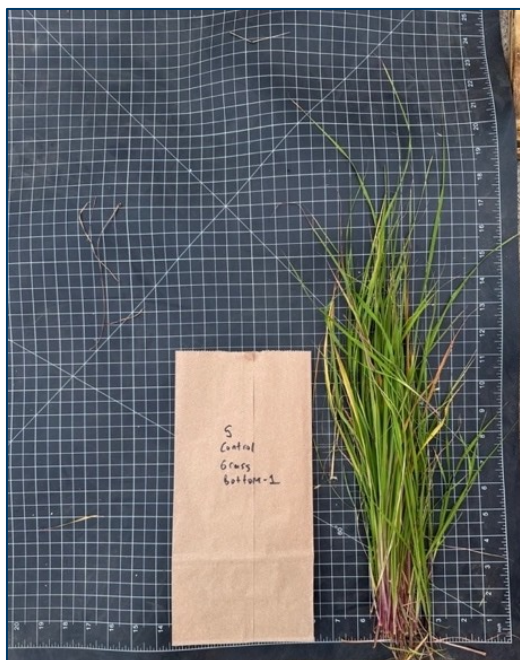
Figure 5.8 Scaled cutting mat used for determining grass heights.
