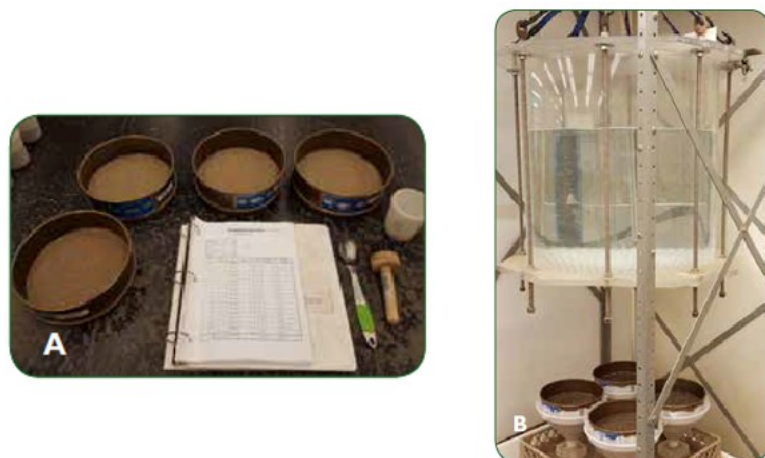
Figure 3.3 (a) Aggregate stability test, (b) A rain-stimulator is used simulate rainfall. (Moebius-Clune et al., 2016)
