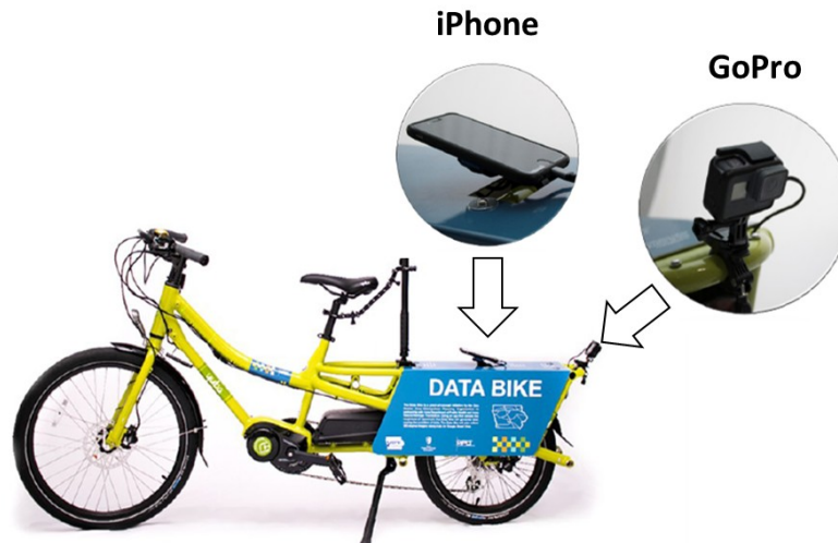
Figure 6-1. Iowa data bike system
