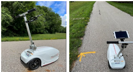
Figure 6-4. Walking profiler used as the reference profiler
