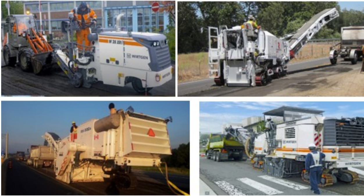
Figure 2-13 Examples of Milling Machines of Different Sizes and Capacities (ASTEC, 2021, Wirtgen, 2021)
