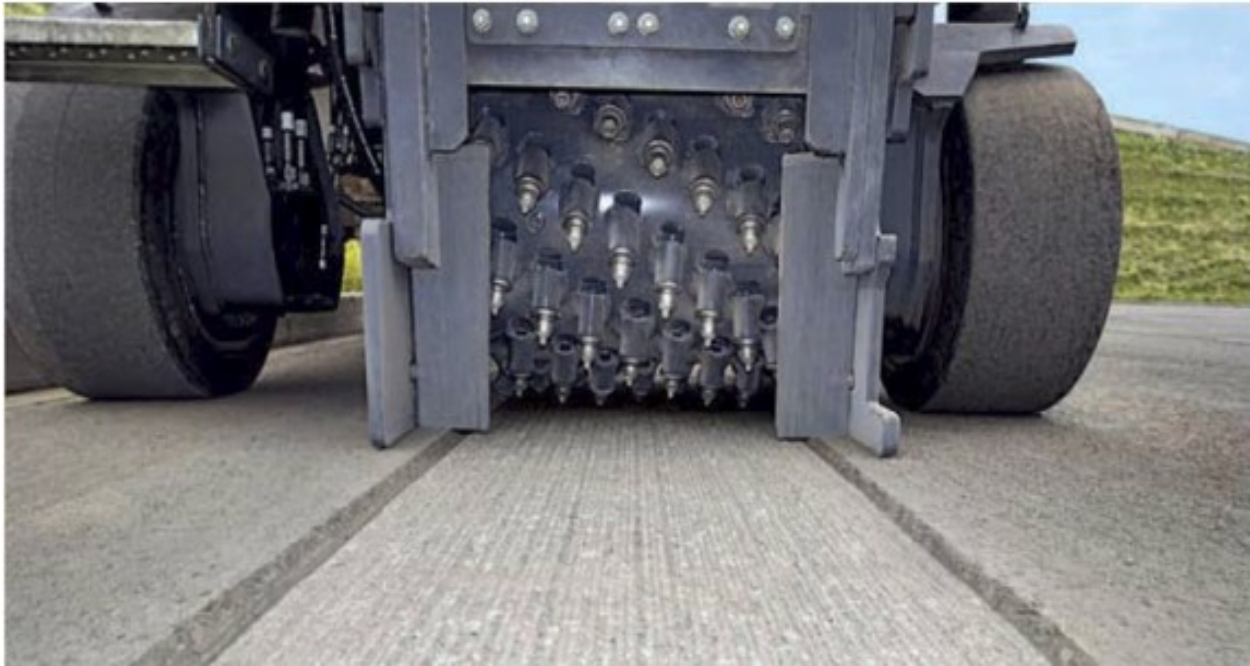
Figure 2-9 Staggered Teeth on the Milling Machine (Wirtgen, 2018)
