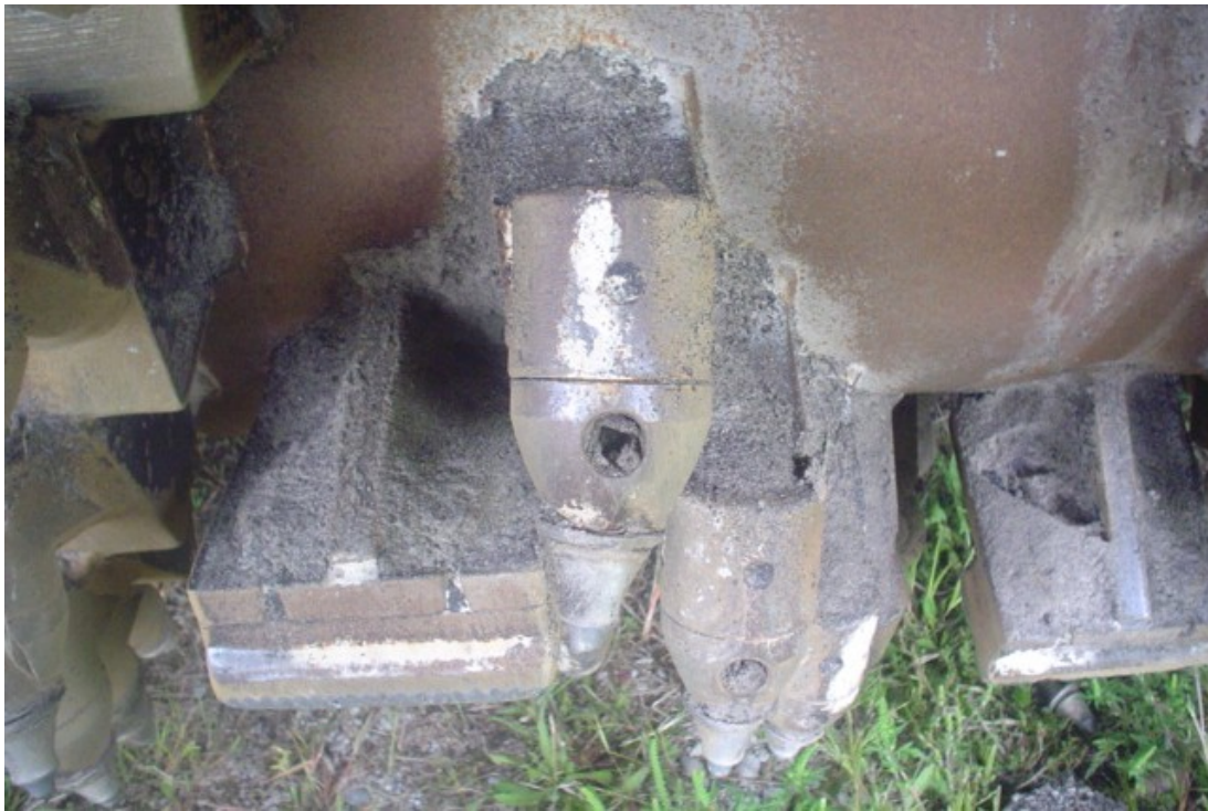
Figure 2-5 Misaligned Tool on Tooth Holder (Hammon, 2015)
