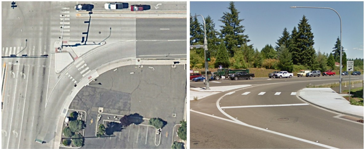
Figure 12. Examples of center-perpendicular crosswalk placement at CRTs [3].
