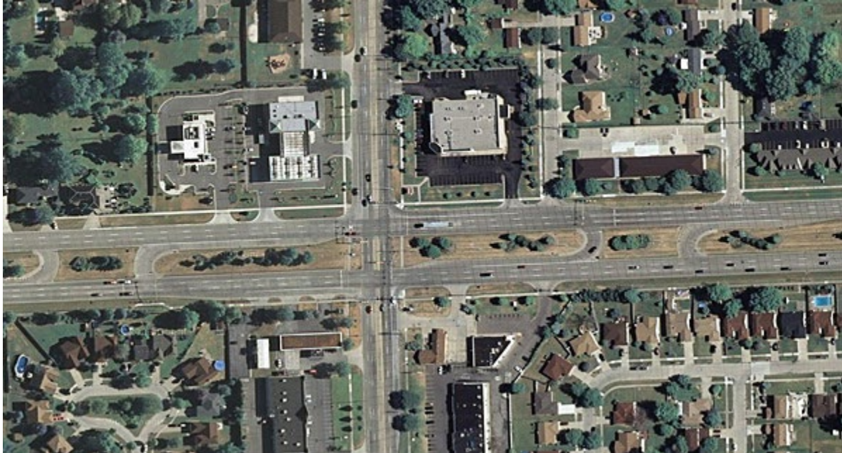
Figure 5.1: Median U-turn intersection
