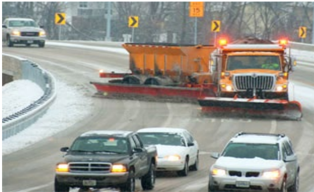
Figure 1.3: Tow Plow in operation
