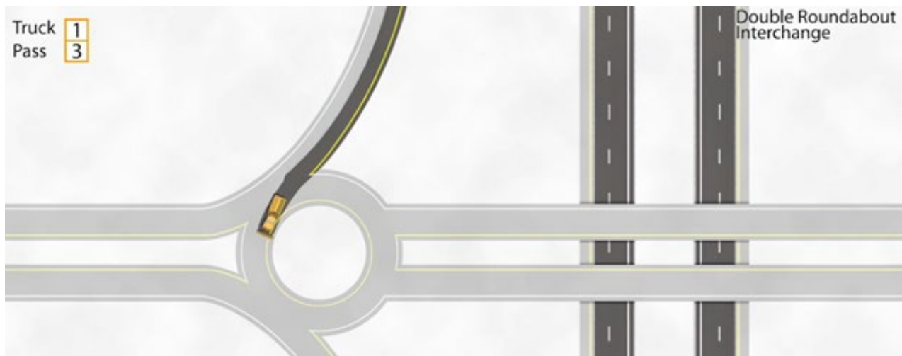
Figure 6.2: snow plowing pattern for the Pass 1/3 (a)
