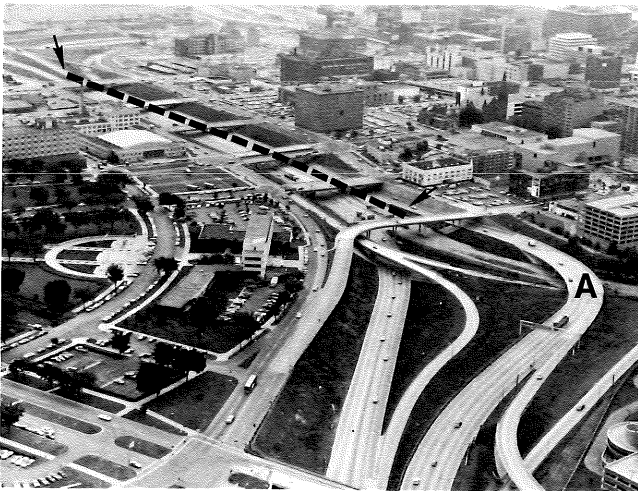
Of concern among traffic engineers are design solutions that will be required for safe and efficient vehicular movement in the common section (dashed line in photo) of I-35E and I-94 between the St. Paul business district and state capitol complex if a direct interstate connection is provided for a roadway in the "Pleasant Avenue Corridor." The probable site of a direct connection is shown by the letter "A" in the aerial view.
