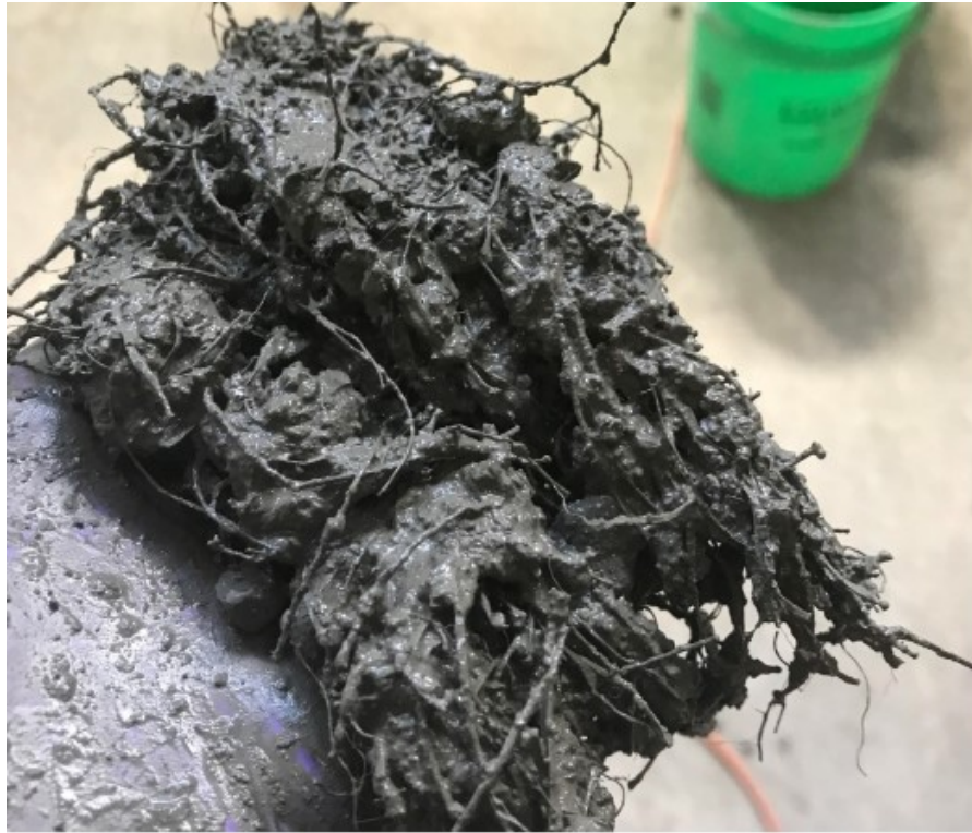
Figure 3-11. Fiber Balling of Fiber 1 (Twisted Geometry)
