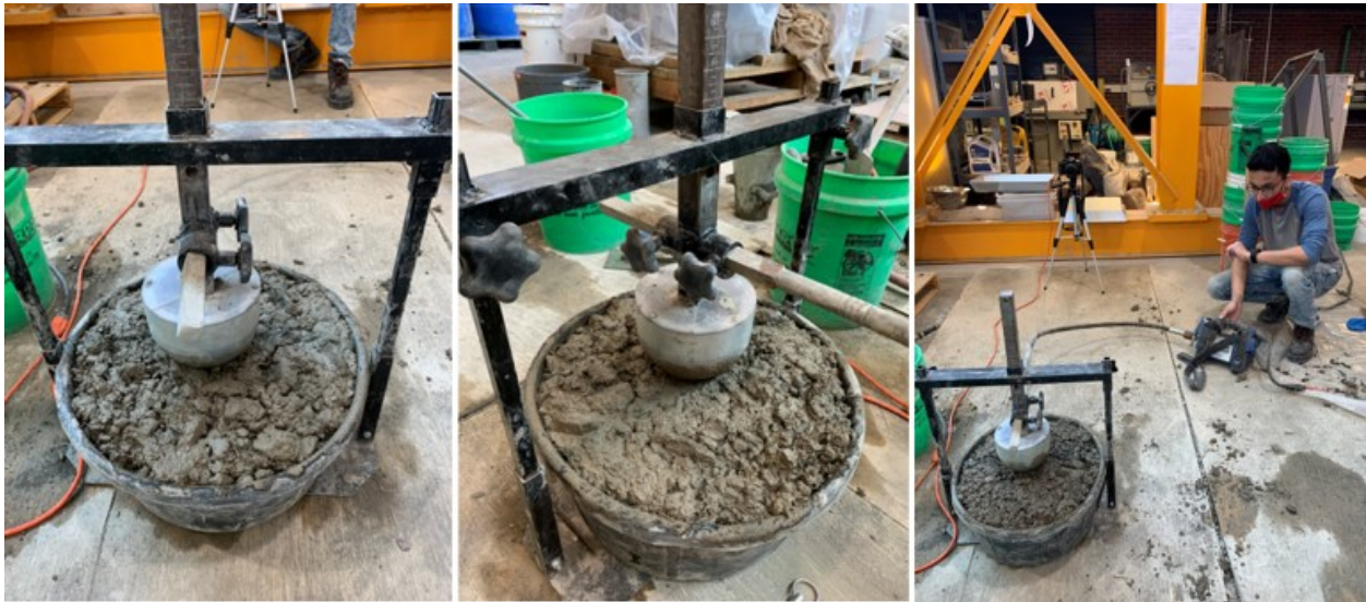
Figure 3-14. V-Kelly Test in Process
