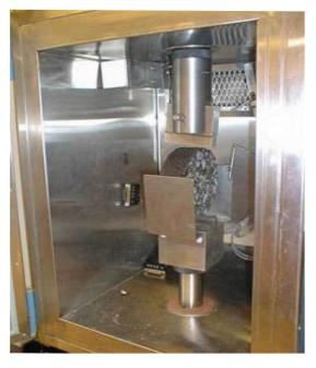
One promising performance test is the indirect tensile strength test, which can be used to measure tensile strength by applying a load across the diameter of a cooled, cylindrical specimen and increasing the load until the specimen fractures.
