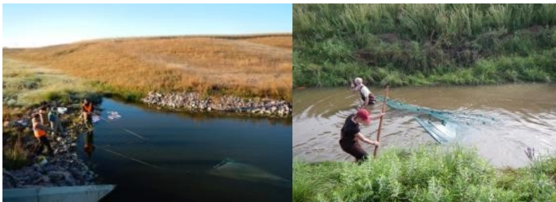
Figure 2.9 Deployment of the mini-Missouri trawl in the in a deep pool, and bag seine in a shallower stream reach.
