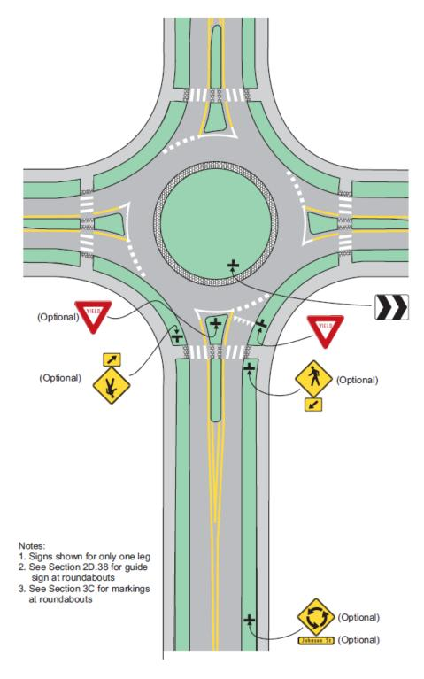
Figure 2.3 Example of regulatory and warning signs for a one-lane roundabout. (3)
