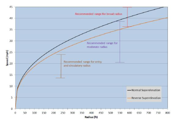
Figure 3.15 Radii-Speed relationship for chicane design (15).
