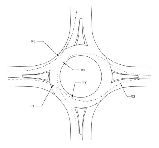
Figure 2.1 Fastest vehicle path radii. (1)
