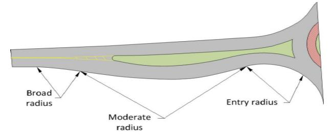
Figure 3.14 Example of chicanes at roundabout approach (15).
