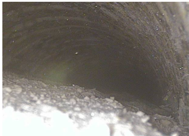
Figure 8.11. Borescope picture looking toward low point in tendon 1
