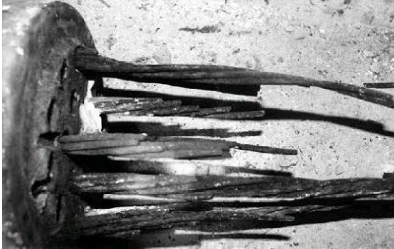
Figure 2.2. Strands corroded at anchor (Corven Engineering, 2002)
