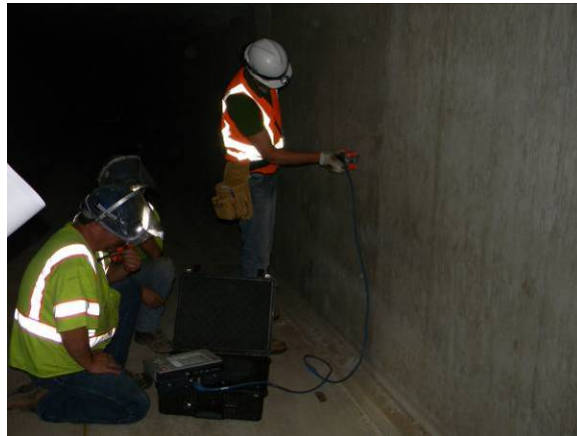
Figure 3.1. Ground penetrating radar in box girder
