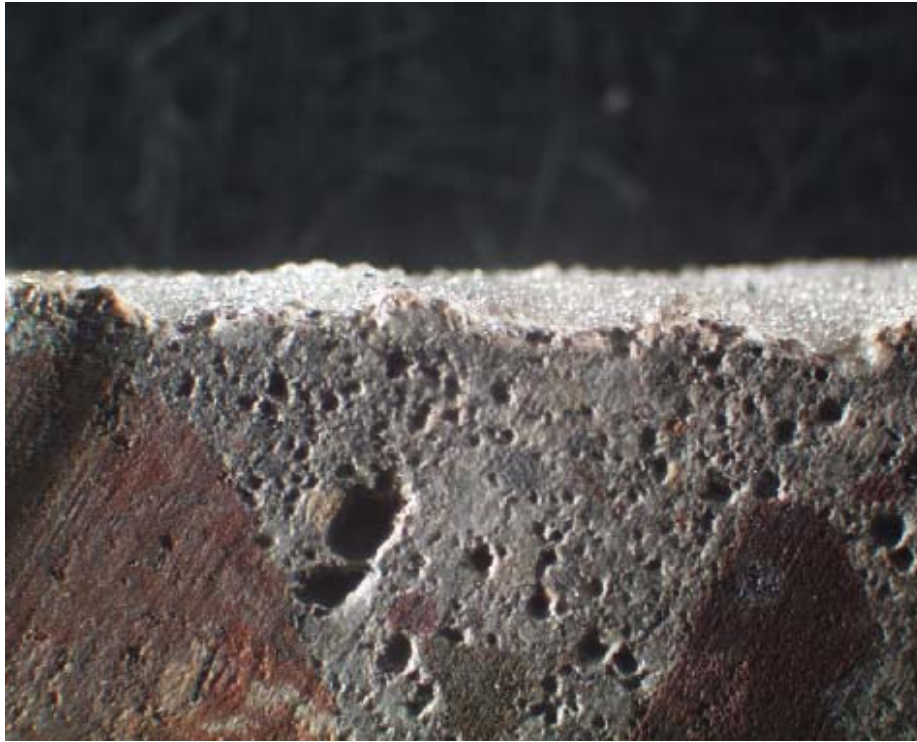
Figure 2.4. Petrographic slice of Astro-turf textured pavement
