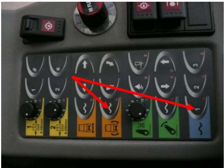
3. Activate the float position of both the 3-point hitch and the tilt function
