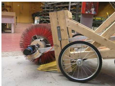
Figure 23: Working prototype – Lifting tines details
