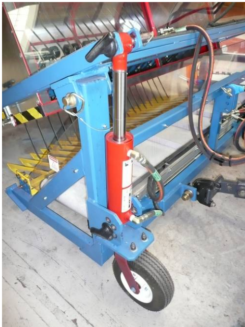
Figure 33: Supporting wheels and skid plates
