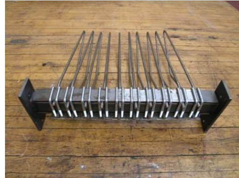
Figure 23: Working prototype – Lifting tines details
