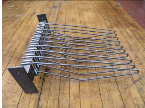
Figure 23: Working prototype – Lifting tines details
